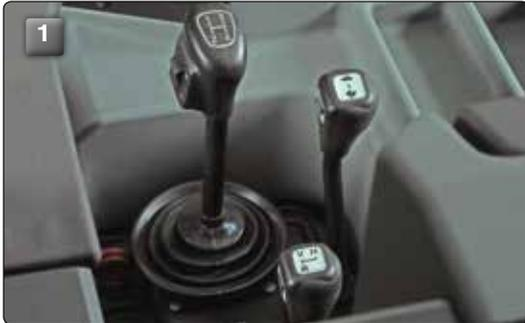
Depending on the work, the operator can choose between the **speed change gearbox (1)** and the **continuously variable gearbox (2)**. Switching is done by a control lever.
