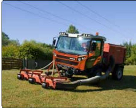
The hydrostatic drive makes safe starting and stopping possible even on extremely steep slopes, taking the driver and vehicle safely through everyday work.
