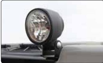
One or two **working lights behind** the cab provide sufficiently good visibility at night.
