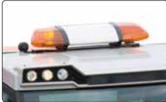
The **optical warning system** can be mounted on the roof of the Muli and can be labelled individually.
