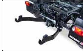
The **rear 3 point linkage** is equipped with fixed category 2 lower links.
