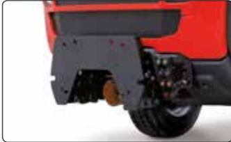
The device **mounting frame** allows front attachments to be directly mounted, e.g. snow plough or blower.
