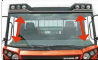
The roof of the Muli T10 X can accommodate up to 3 working lights per side or a **changeable lighting** for use with front attachment.
