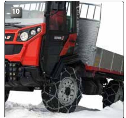
The 360° pivoting **central joint (10)** between front and rear axles makes sure that all 4 wheels have permanent ground contact, ensuring safe driving behaviour in any situation. It gives you full power transfer and optimum soil protection, even in rough terrain.
