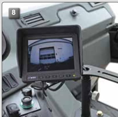
Many attachments have their own control unit or display (e.g. reversing camera). They can be ideally placed in the Muli cab by means of a specially developed **monitor holder (8)**. Cables between the attachment and control unit can be routed neatly and with a minimum of space into the cab through a cable lead-through in the tailboard. Pulse or power outlets for attachments are available as options.
