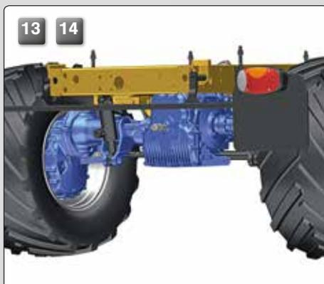
The front and rear axles are designed as **portal axles (13)**. This design provides the largest possible ground clearance with the corresponding passage width between the wheels. The ground clearance is 450 mm.
