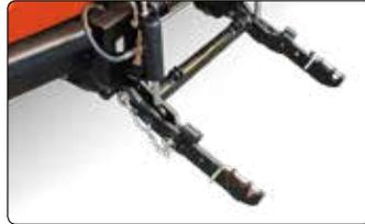
The **front 3 point linkage** with forks is available with electro-hydraulic weight compensation and vibration damping.
