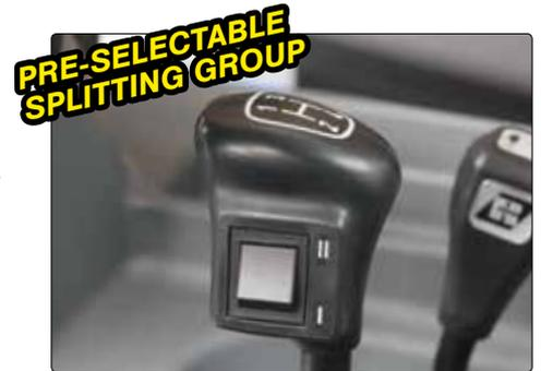
The 8 forward gears are subdivided at the push of a button into 16 gears by the splitting ("half gear") group, creating an even finer speed stepping.
