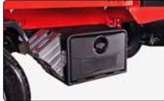
The splash-proof and lockable **tool box** made of polyethylene provides enough storage space for straps, tools or options.
